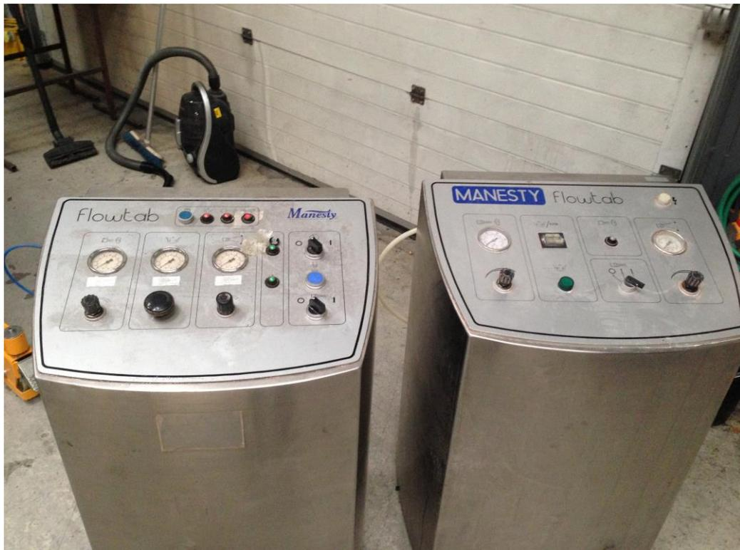
We have 2 Flowtabs available designed for a 150 or 75 size machine and capable of driving up to 3 nozzles
