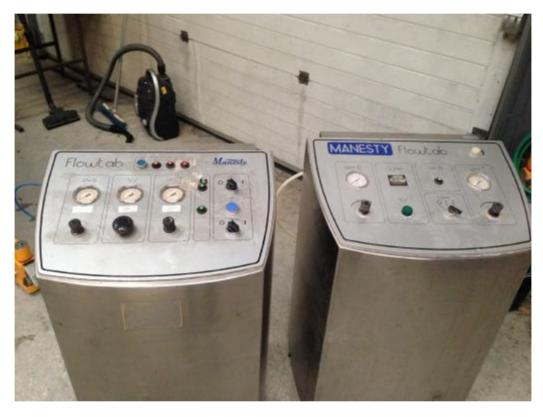
We have 2 Flowtabs available designed for a 150 or 75 size machine and capable of driving up to 3 nozzles
